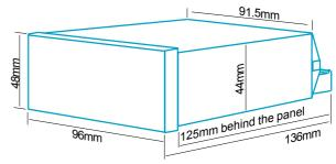
Panel cutout should be 92mm wide x 45mm high, +1mm, -0mm 1/8 DIN. Depth behind panel 125mm max, including cables. 350 grammes typical weight
